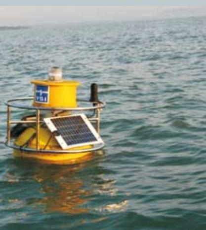
The state of the art sensors are being procured from YSI, USA, a global leader in manufacturing of the sensors used by USGS, NOAA and the leading laboratories world over. These are equipped with technology to prevent bio-fouling by using an automated wiper. A calibration unit has been established by the company at WRTC. The calibrated sensors would be swapped at each location at an interval of three weeks.
