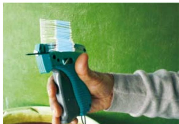
Tagging gun loaded with a clip of numbered tags.
