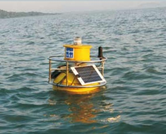
The state of the art sensors are being procured from YSI, USA, a global leader in manufacturing of the sensors used by USGS, NOAA and the leading laboratories world over. These are equipped with technology to prevent bio-fouling by using an automated wiper. A calibration unit has been established by the company at WRTC. The calibrated sensors would be swapped at each location at an interval of three weeks.
