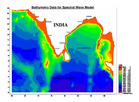
Bathymetry considered for Spectral wave Model
