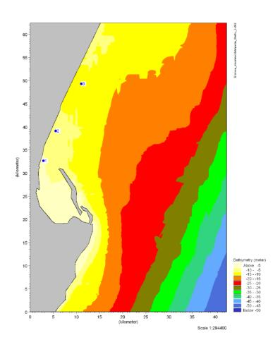
Bathymetry considered for near-shore spectral wave model
